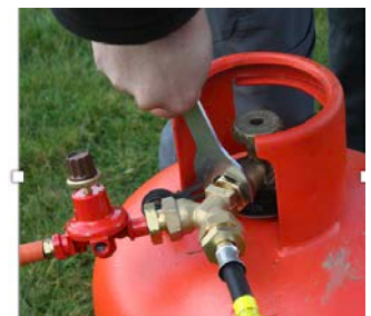
8. Use the spanner to tighten the fixings on both cylinders. Make sure they are firm. Do not over tighten.
