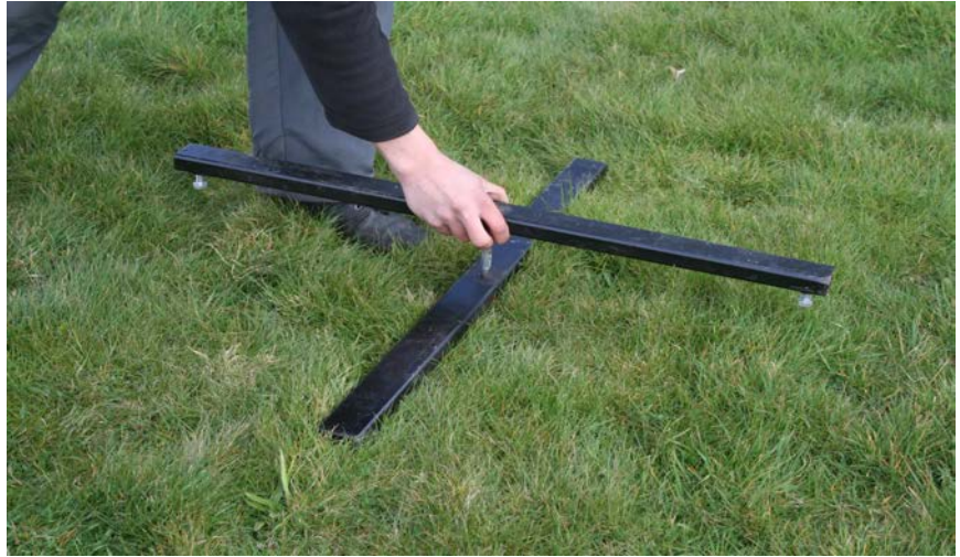
2. Set up base. If on grass, secure base using steel pins. If on roof top or hard standing, use sandbags or concrete blocks for additional stability. 3. Use a small spanner to adjust the feet if sitting on hard standing, pavements, roof tops etc to enhance stability
