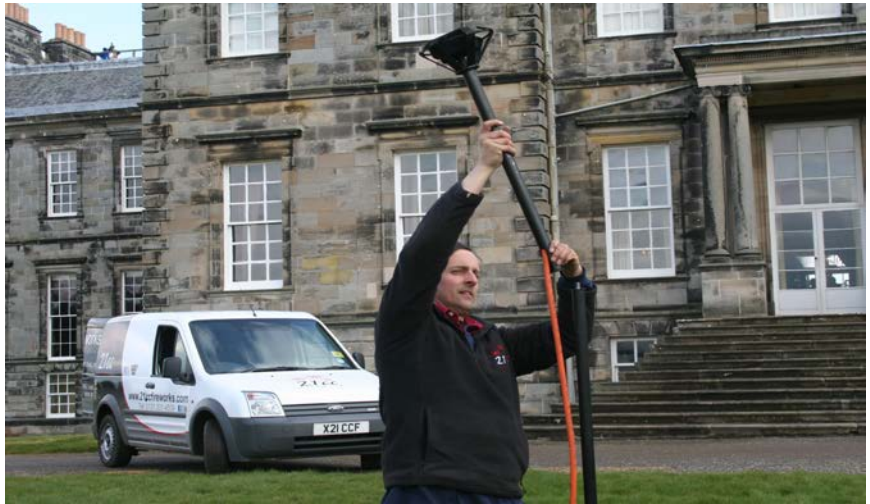
5. Screw the top pole onto the bottom pole. Ensure all sections are fixed firmly.
